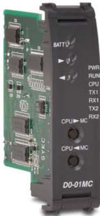
Modbus RTU master/slave communication to GS1 AC drive
